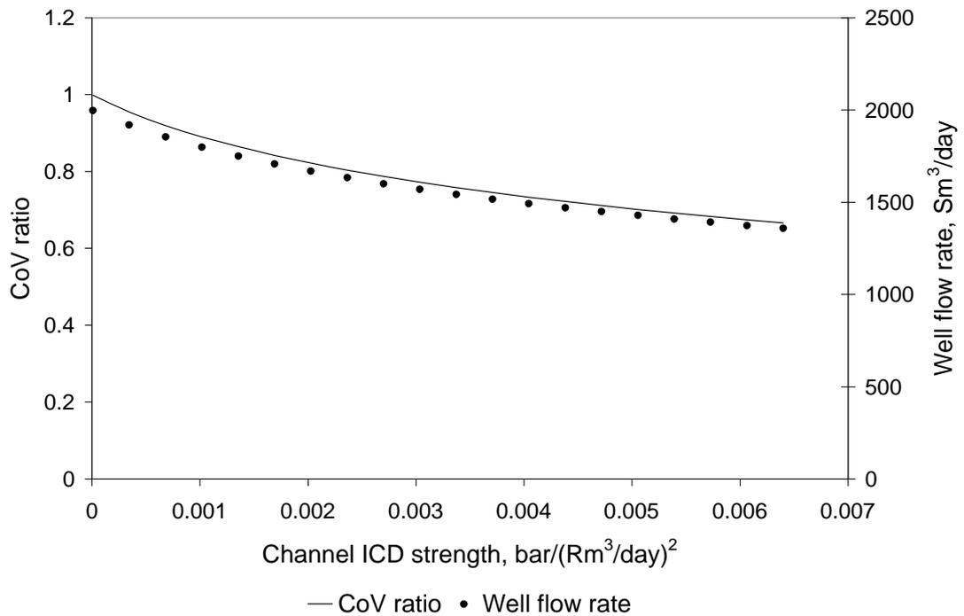
Figure 6.4: Dependence of inflow equalisation and well productivity on ICD strength for *channel* ICDs in a *medium* productivity reservoir
