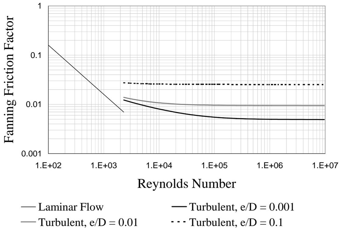
Figure 4.1: Fanning friction factor for rough pipes (Haaland's correlation)
