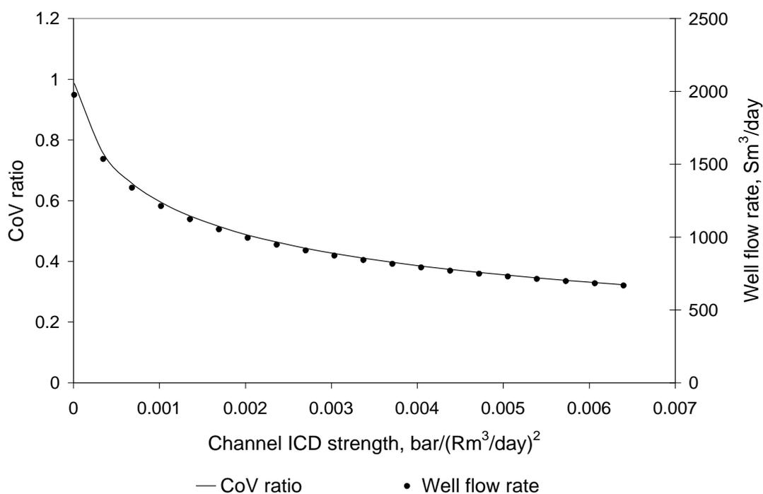
Figure 6.2: Dependence of inflow equalisation and well productivity on ICD strength for *channel* ICDs in a *highly productive* reservoir
