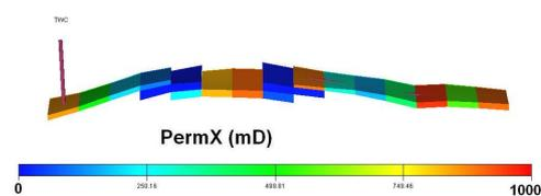
Figure 3.7: Permeabilities of the grid blocks connected to the well
