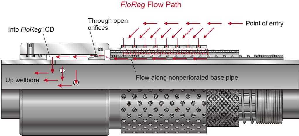
Figure 1.3: Orifice ICD schematics (courtesy Weatherford)
