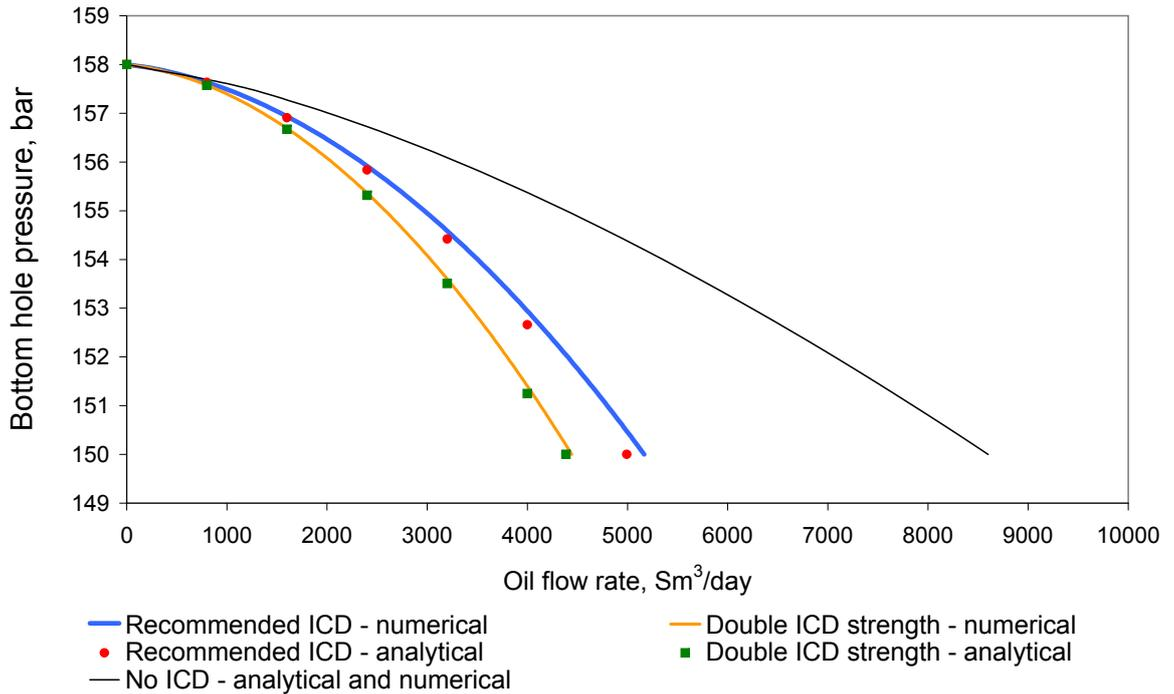
Figure 5.4: Impact of the “recommended ICD” on well’s IPR
