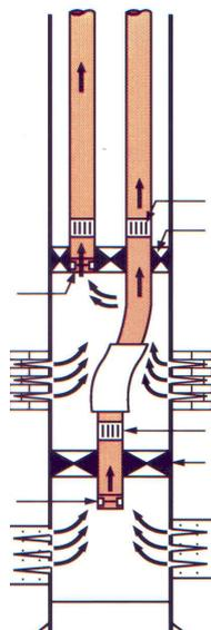
Figure 2.8: Multiple layer reservoir management with dual completion
