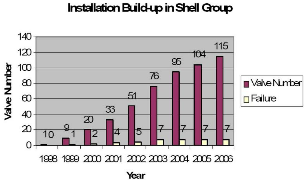
Figure 2.10: ICV reliability statistics for all-hydraulic systems (de Best and van den Berg, 2006)
