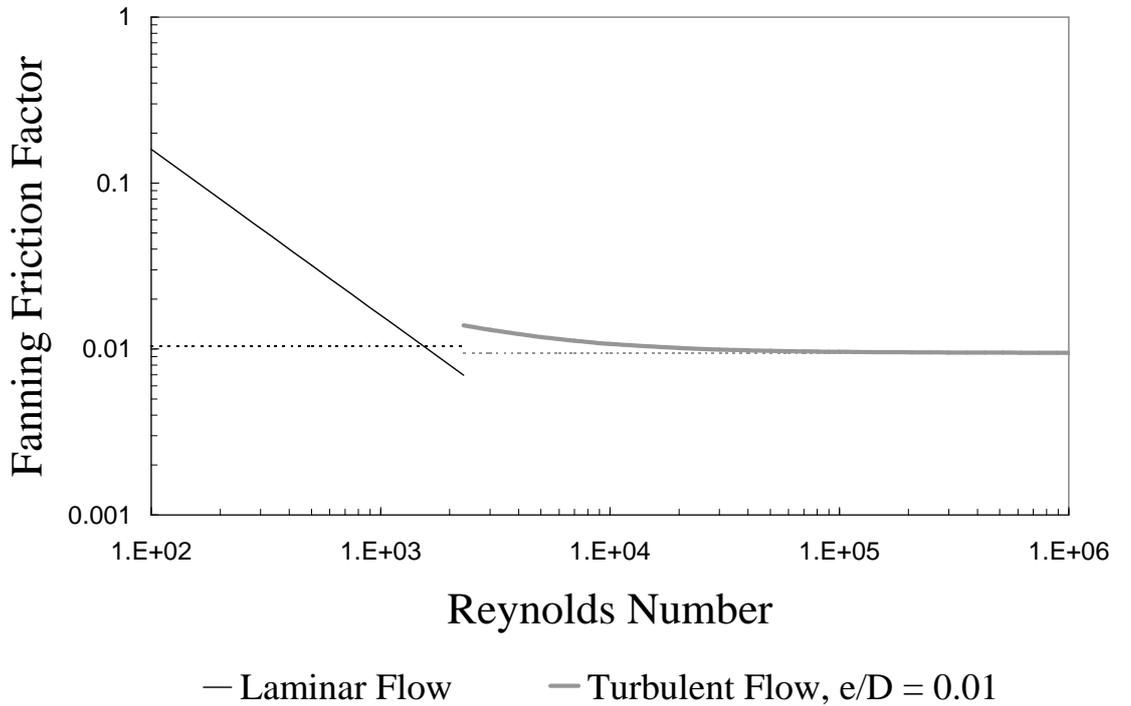
Figure A.2: Averaging the friction factor for rough pipes
