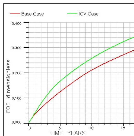
Figure 3.3: Increase in recovery for non-optimal well location
