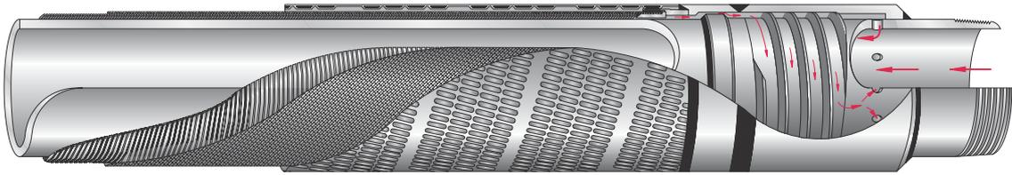
Figure 1.2: Channel ICD schematics (courtesy Baker Oil Tools)
