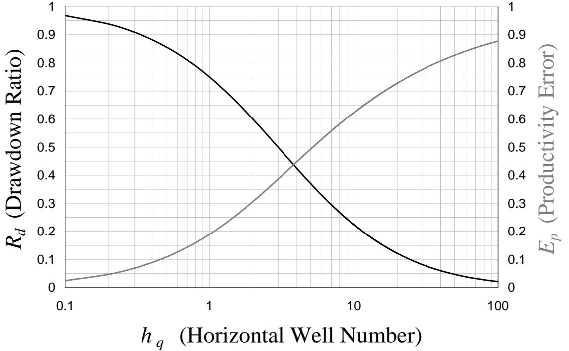
Figure 4.5: The drawdown ratio and the productivity error for a *rate* constrained well
