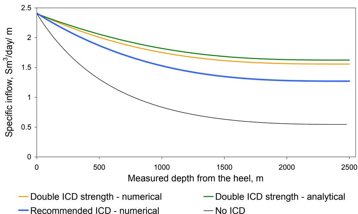
Figure 5.2: Impact of the “double ICD” strength on the specific inflow distribution for the Troll case
