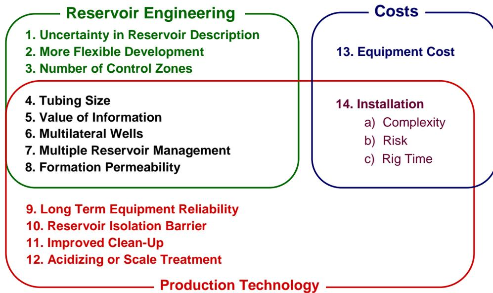
Figure 2.1: ICV vs ICD comparison framework for oil field applications
