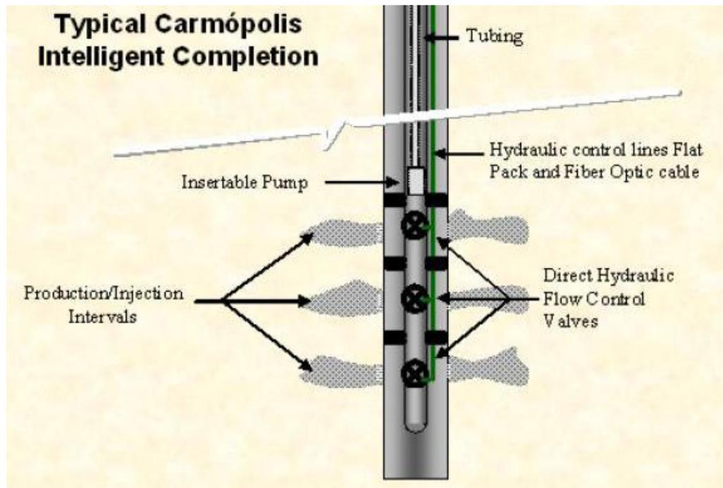
Figure 2.9: Multiple layer reservoir management with single string ICV completion (Silva et al., 2005)
