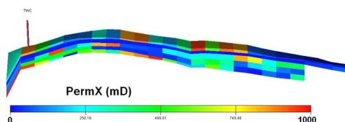
Figure 3.6: Vertical slice of reservoir at optimal well location
