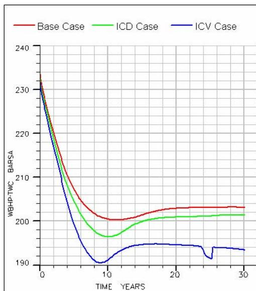
Figure 3.9: Flowing bottom hole pressure comparison for one of the 8 realisations
