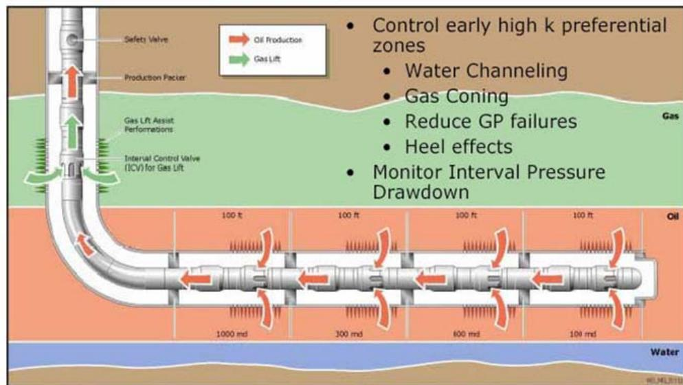
Figure 1.1: Schematics of intelligent well (courtesy WellDynamics)
