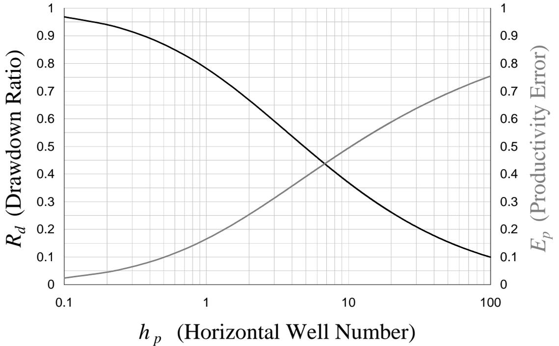
Figure 4.6: The drawdown ratio and the productivity error for a *pressure* constrained well
