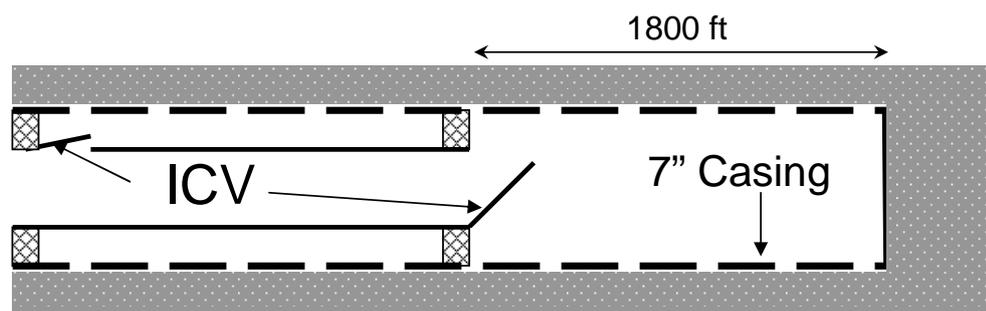
Figure 2.3: A two-zone ICV completion
