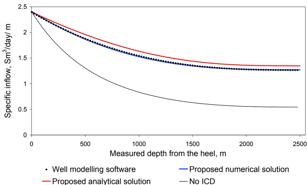
Figure 5.1: Impact of the “*recommended ICD*” on the specific inflow distribution for the Troll case
