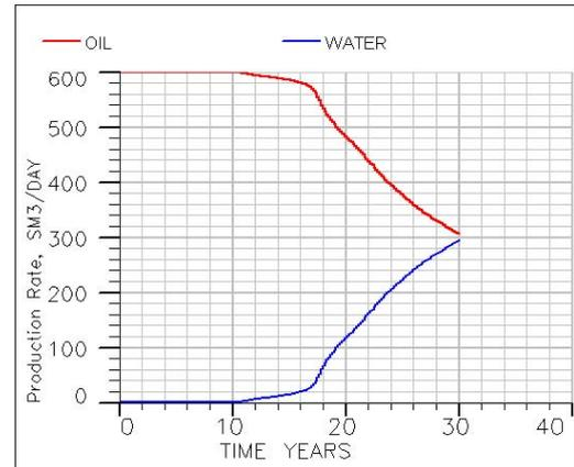
Figure 3.5: Oil and water production for optimal well location
