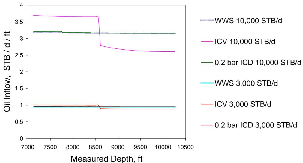
Figure 2.6: Medium Permeability case, inflow from reservoir to well
