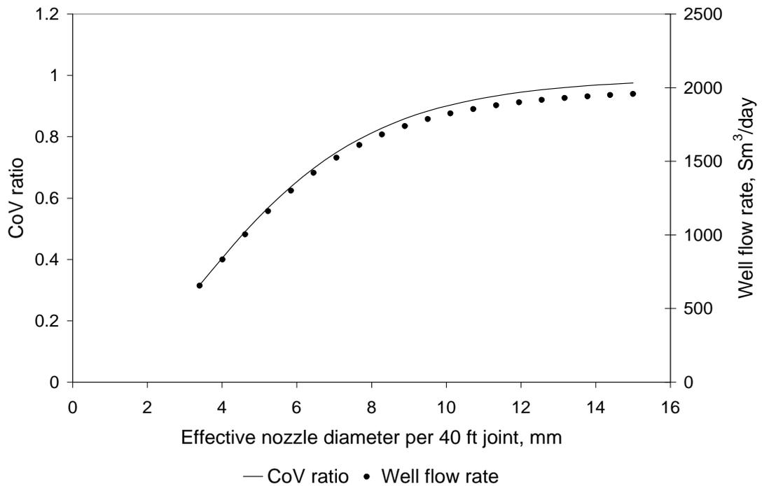
Figure 6.3: Dependence of inflow equalisation and well productivity on ICD strength for *nozzle/orifice* ICDs in a *highly productive* reservoir
