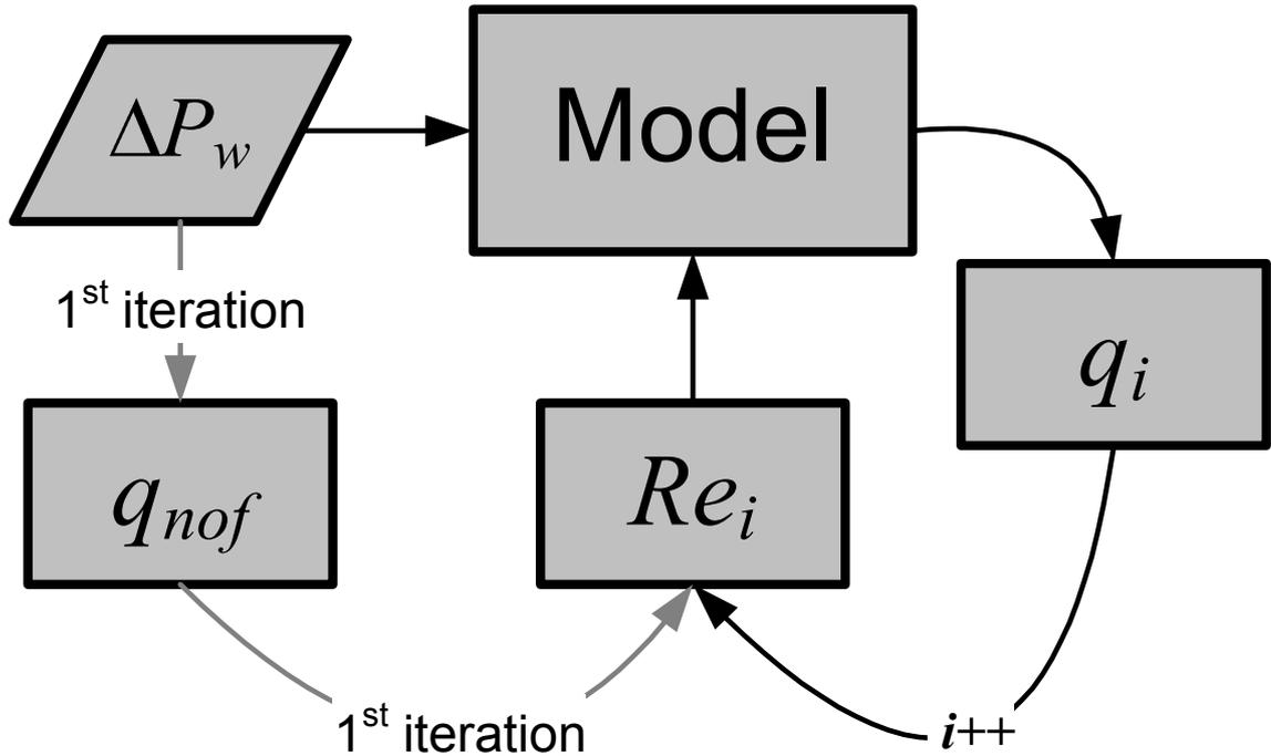
Figure A.1: Reynolds number calculation for a pressure constrained well
