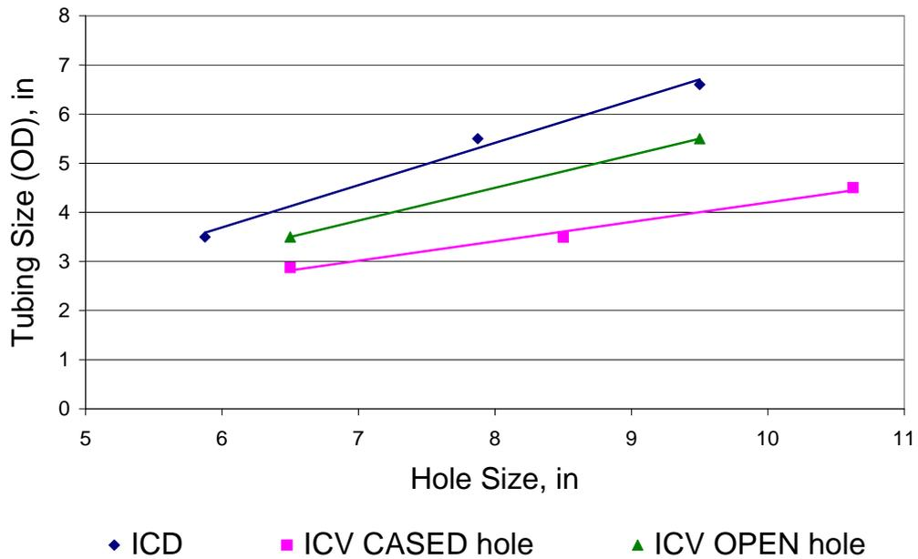
Figure 2.2: ICD and ICV tubing sizes vs wellbore hole size
