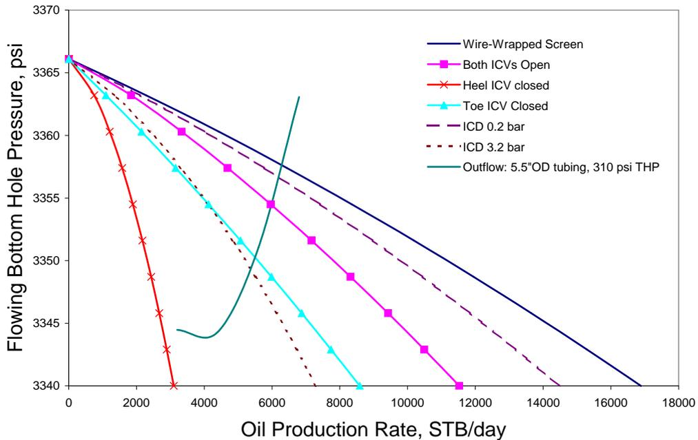
Figure 2.7: High Permeability case, impact of advanced completions on inflow performance
