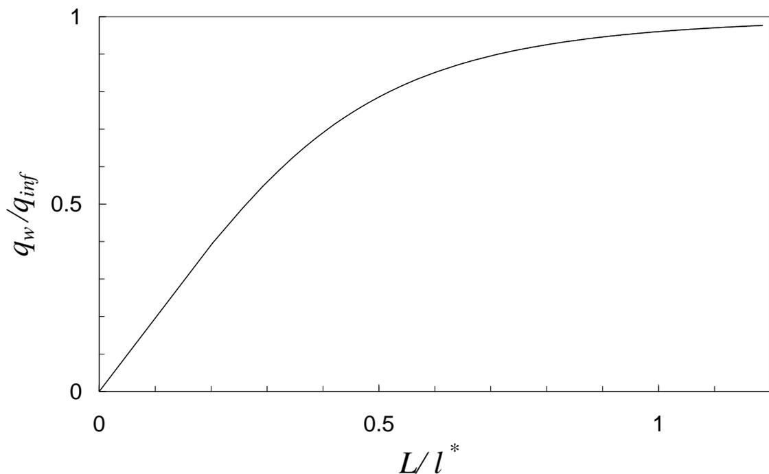
Figure 4.7: The dependence of well rate on completion length
