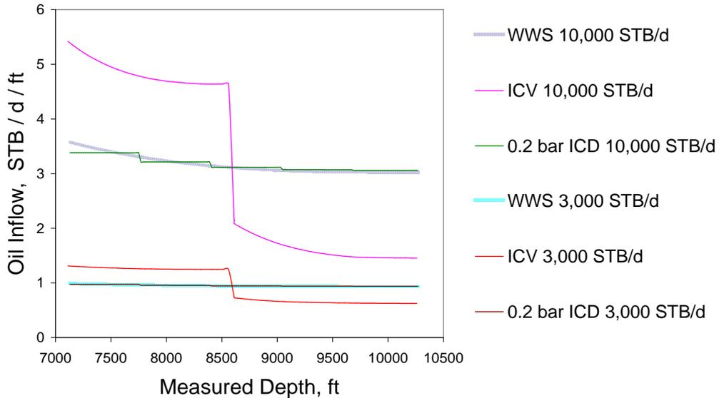
Figure 2.4: High Permeability case, inflow from reservoir to well
