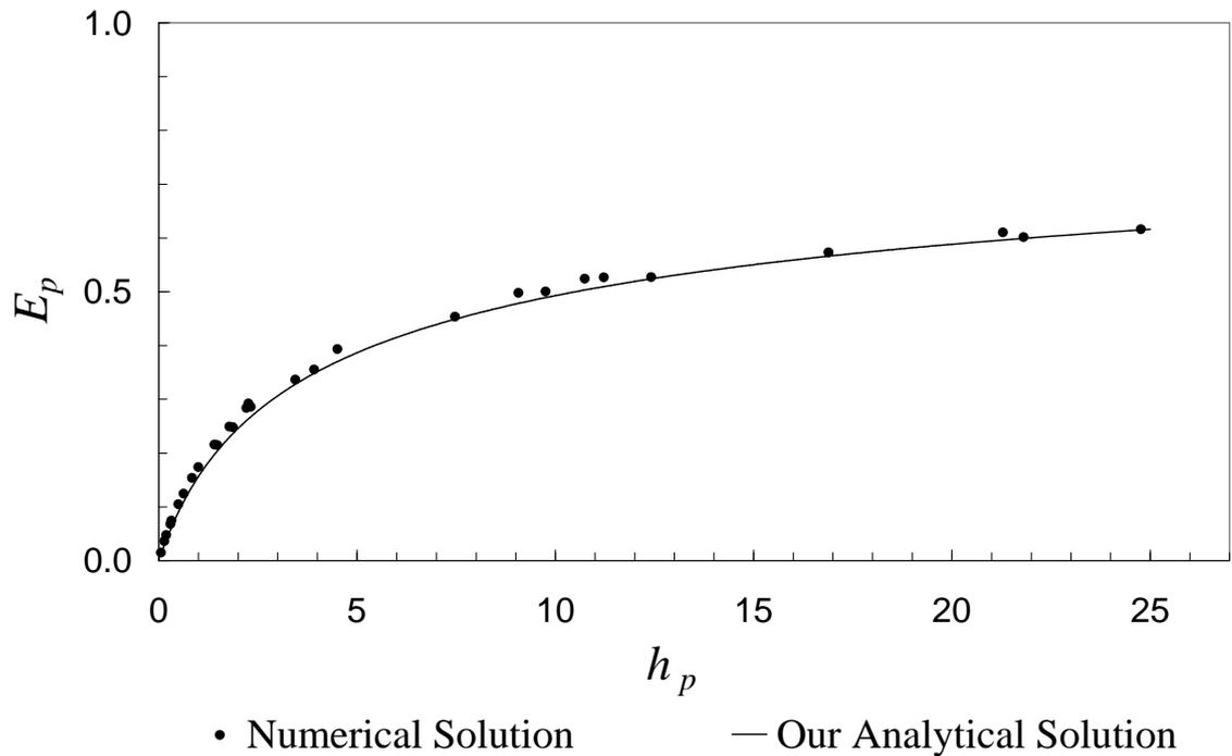
Figure 4.9: Numerical verification of Formula (4.57) for the productivity error,  $E_p$ , of a pressure constrained well
