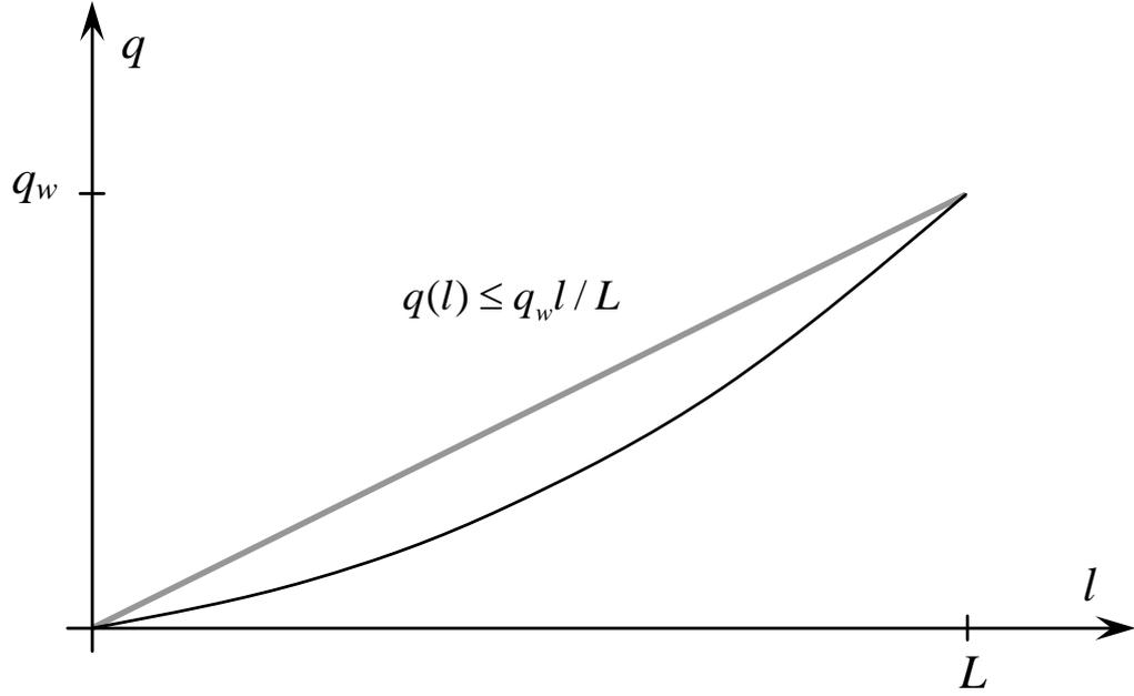
Figure C.1: Upper estimate of flow distribution along the completion interval
