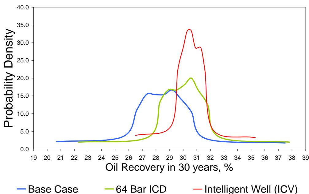
Figure 3.11: Impact of advanced completion on production forecast
