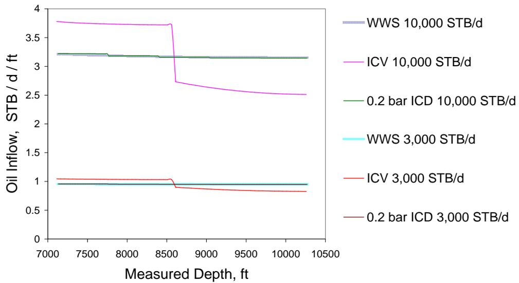
Figure 2.5: Heavy Oil case, inflow from reservoir to well
