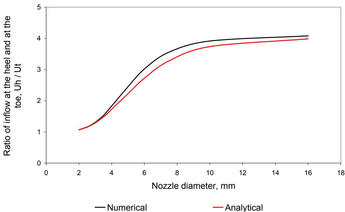
Figure 5.3: Dependence of inflow equalisation on ICD nozzle diameter
