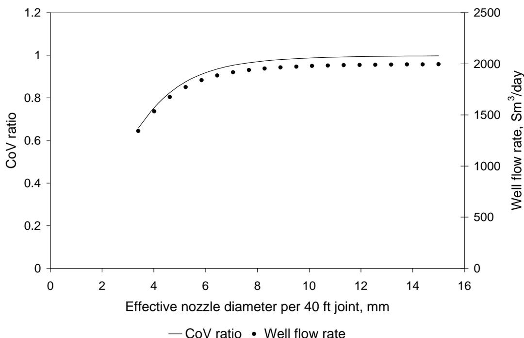
Figure 6.5: Dependence of inflow equalisation and well productivity on ICD strength for *nozzle/orifice* ICDs in a *medium* productivity reservoir
