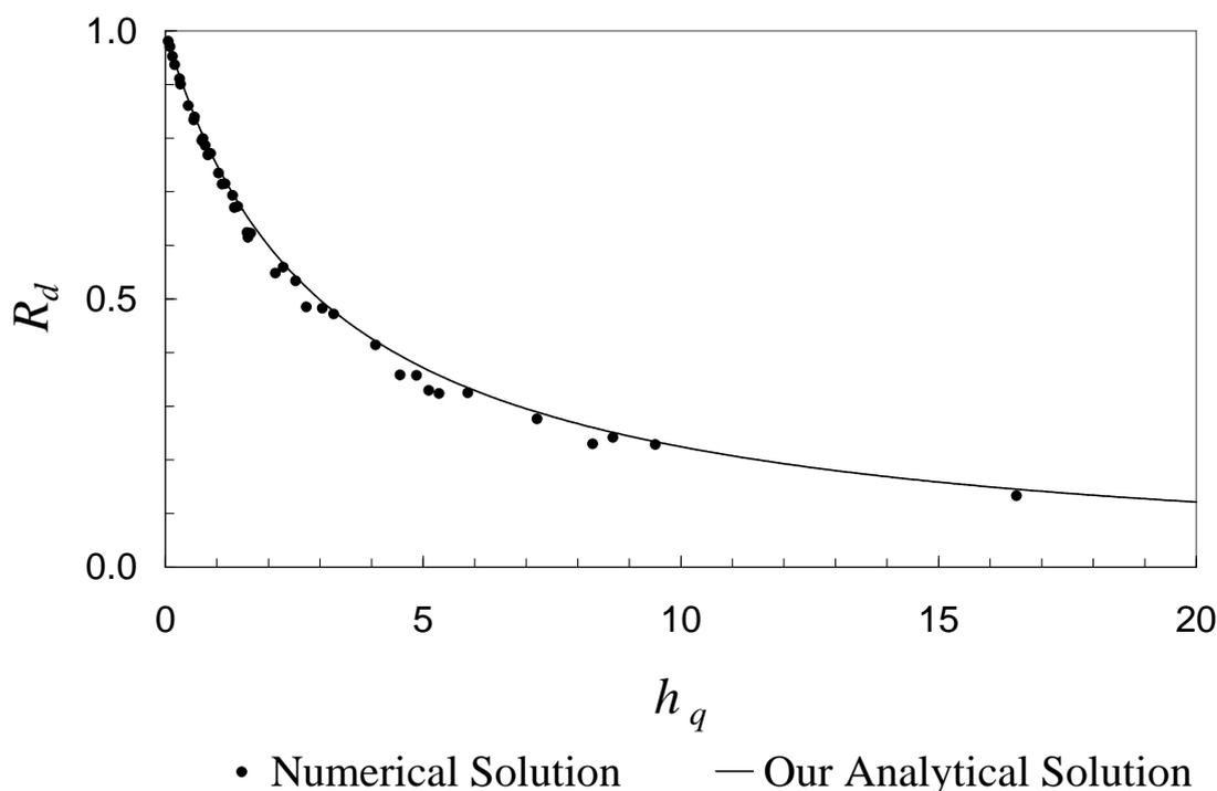
Figure 4.8: Numerical verification of Eq. (4.47) for the drawdown ratio,  $R_d$ , in a rate constrained well.
