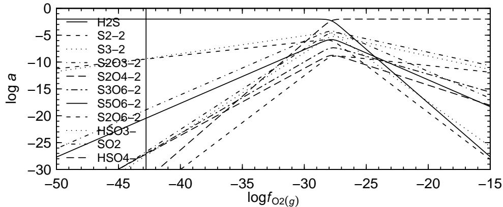
The first diagram is very similar to the one shown by Seewald, 1997, but the second (where we have set `residue=TRUE`) is quite different. There, the function was told to rewrite the formation reactions of the aqueous sulfur species for their residue equivalents (where the number of “residues” in each species is the coefficient of the immobile component, in this case H<sub>2</sub>S, in the formation reaction) in the same way the formation reactions for the proteins were rewritten above.
